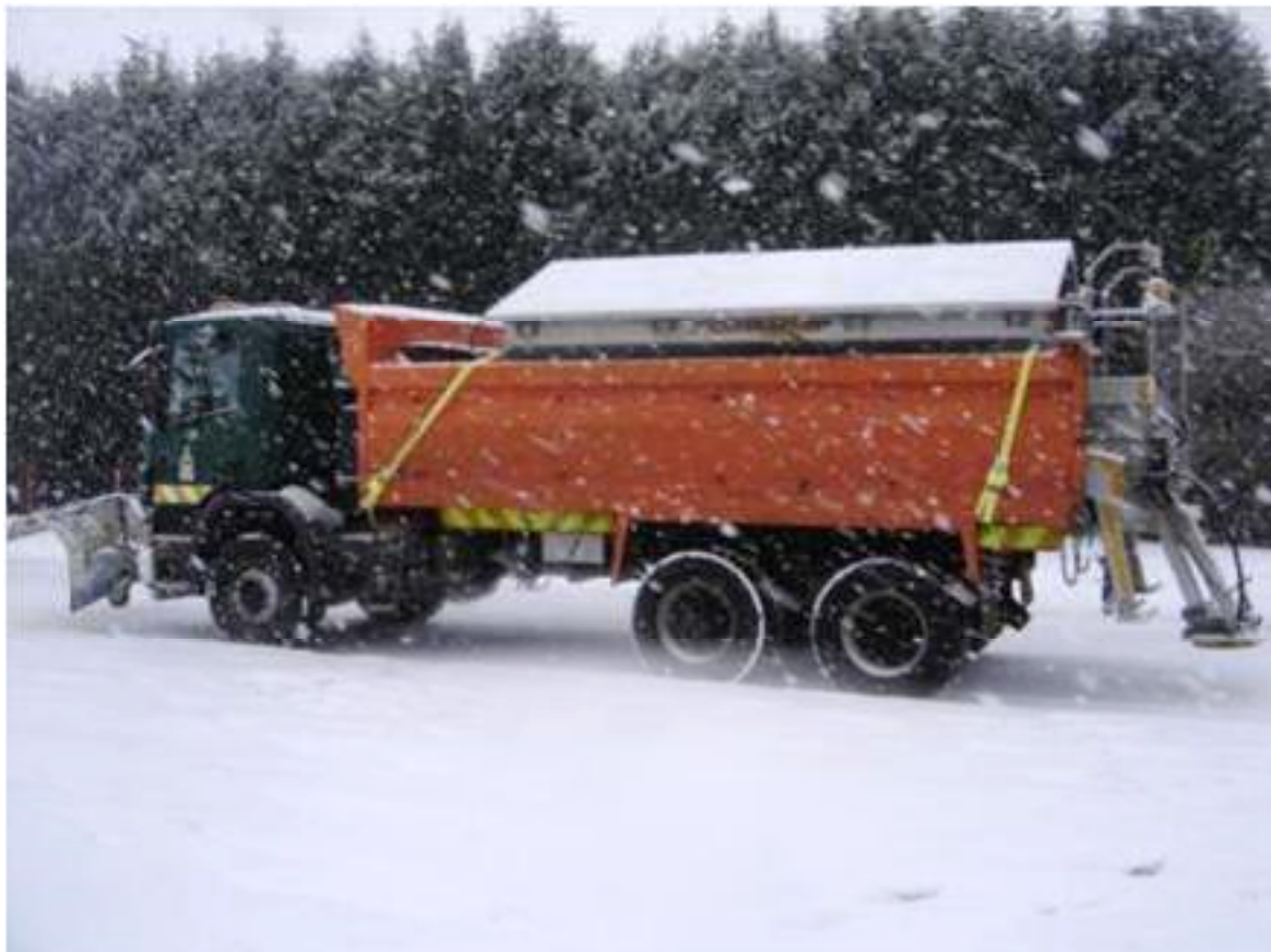
Figure 1: Demountable salt spreader
