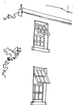
Sketch 10: Inappropriate uPVC windows with outward opening has replaced traditional hardwood sliding sash windows. Where possible original windows and doors should be conserved or re-instated.
