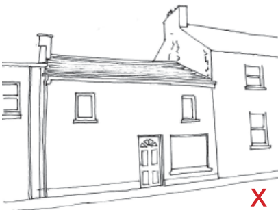
Sketch 7: Solid to void ratio refers to the proportion of the facade that is solid wall versus openings such as windows and doors. In this example the area of facade that is solid is excessive and results in a poor design.
