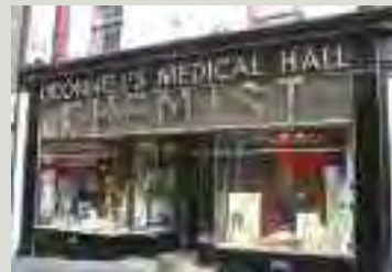
While traditional timber shopfronts are often valued, there is also a legacy of Art Deco-style steel and Vitrolite fronts that should be equally treasured as they represent the modern spirit, new materials and design ethos of their time, illustrated in this elaborate example
