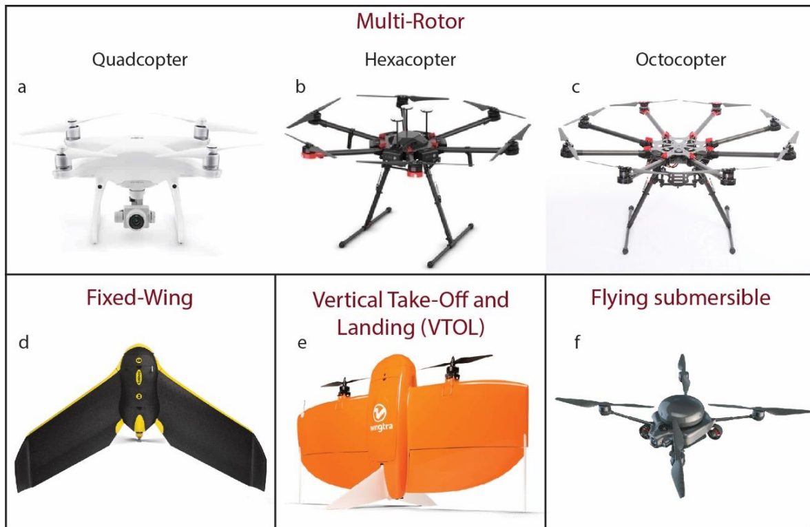
Figure 3: Four types of aerial drone platforms, including three types of multi-rotor systems. (a) DJI Phantom 4 Pro Quadcopter (from c. €1,300) [Source: DJI]; (b) DJI Matrice 600 Pro Hexacopter (from c. €5,699)[Source: DJI]; (c) DJI Spreading Wings S1000 Octocopter (kit from c. €4,400) [Source: DJI]; (d) senseFly eBee (from c. €22,000) [Source: senseFly]; (e) WingTra One VTOL drone (from c. €19,000) [Source: WingTra]; (f) SeaHawk D4 flying submersible [Source: SeaHawk]
