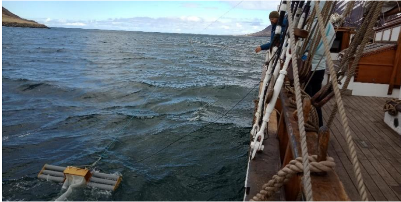
Figure 10 Manta trawl for microplastics, one of the marine science activities on board Opal.
