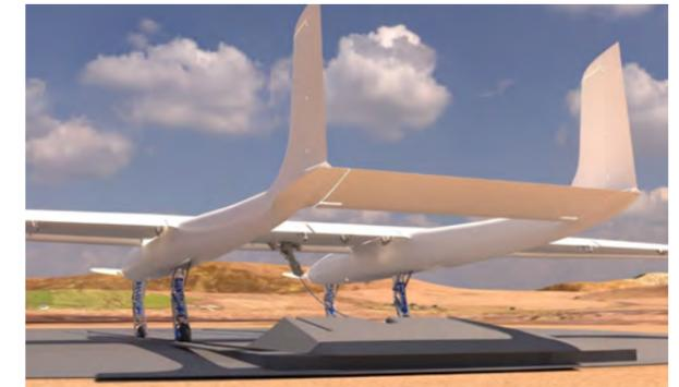
Airborne Wind Energy Systems harness the strong and steady winds at altitudes of several hundred metres. The system proposed consists of a ground-based generator, a launch and land platform and an aircraft-shaped device. The project helps focus the attention of similar energy companies on the natural wind resources of the west of Ireland and places County Mayo to the fore in this area of Research and Development.
