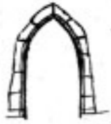
Small pointed recess in nave south wall. (Chamfered sides)
