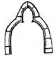
Recess of recess-choir south wall. (Chamfered edges) Pointed.
