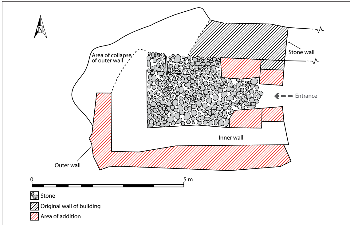
Fig 6.6—Cloonfane: ground-floor plan of double-walled building, with additions marked in red.
