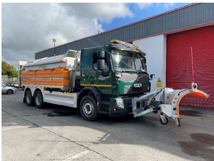
Figure 2: New permanently mounted pre-wet salter
