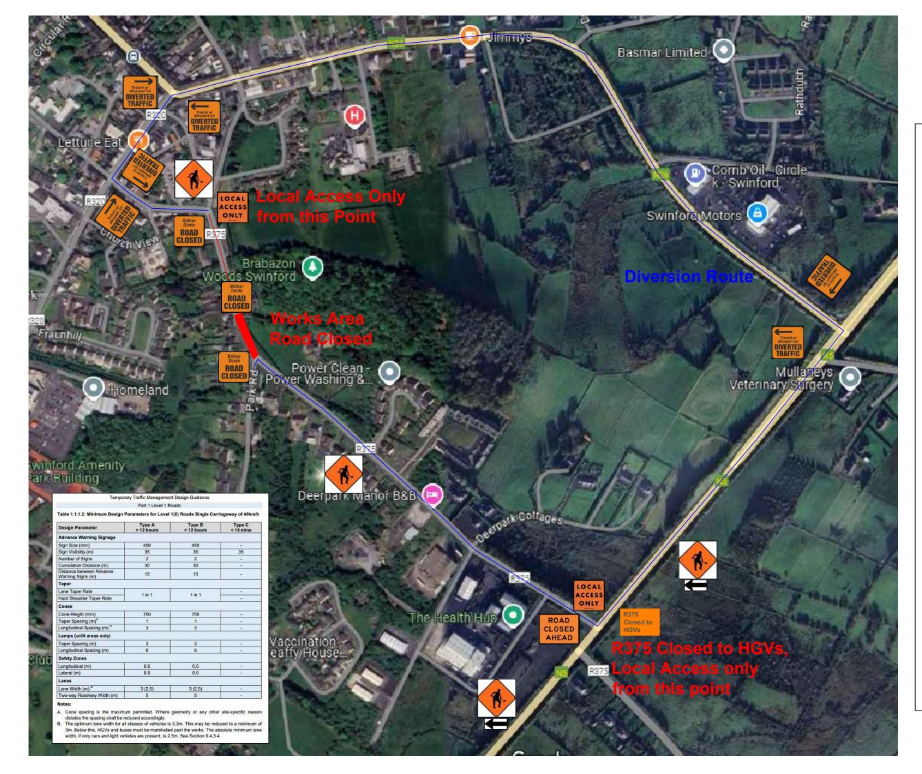
Traffic Management Plan in Accordance with Chapter 8 TSM, TTM Design Guidance, & TTM Operations Guidance
